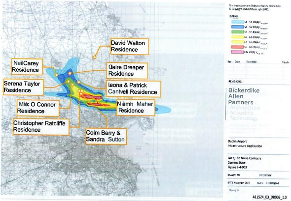
Figure 2: DAA current state noise contour.
